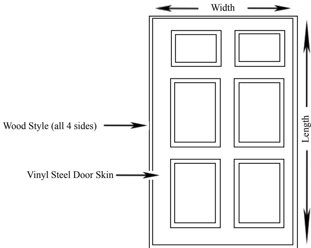
**NOTE: The 7000 Series STR door does not have a folded lip. These doors are flush with the edge of the jamb boards when they are closed.**
