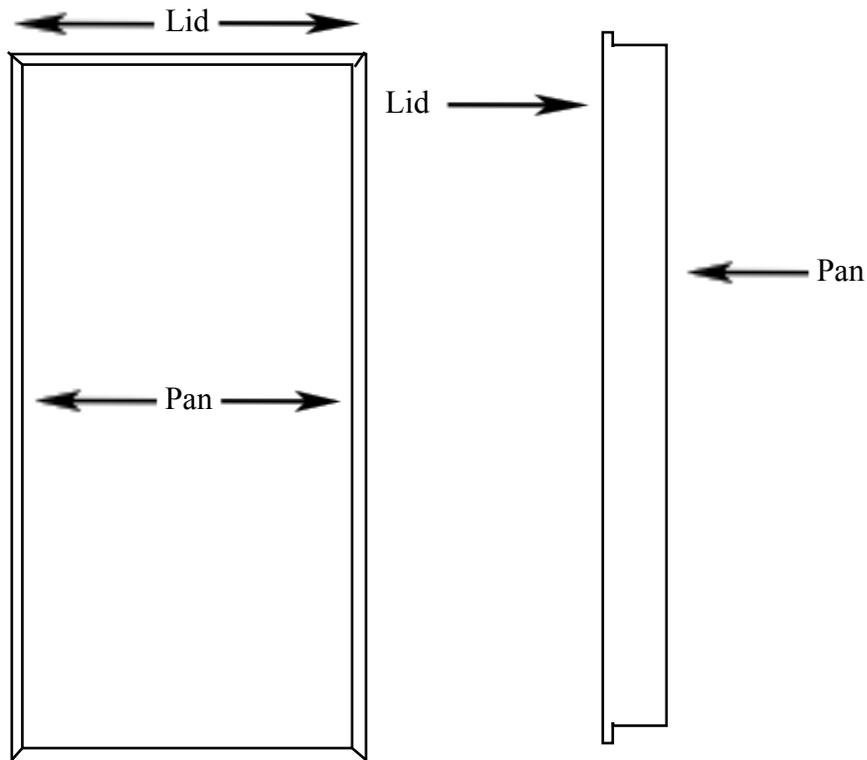
**NOTE:** For regular doors, the lid will be on the outside of the home and the pan will be on the inside (200, 300 & 400 Series). These doors will have aluminum frames.
